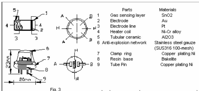
Structure and configuration of MQ136 gas sensor is shown as Fig. 3, sensor composed by micro AL<sub>2</sub>O<sub>3</sub> ceramic tube, Tin Dioxide (SnO<sub>2</sub>) sensitive layer, measuring electrode and heater are fixed into a crust made by plastic and stainless steel net. The heater provides necessary work conditions for work of sensitive components. The enveloped MQ-4 have 6 pin, 4 of them are used to fetch signals, and other 2 are used for providing heating current.
