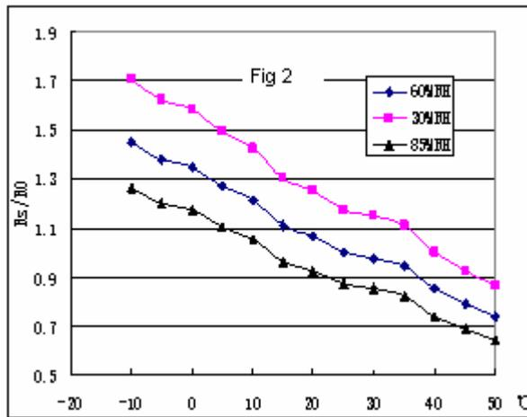
Fig.2 shows the typical temperature and humidity characteristics. Ordinate means resistance ratio of the sensor ( $R_s/R_o$ ),  $R_s$  means resistance of sensor in 50ppm SO<sub>2</sub> under different tem. and humidity.  $R_o$  means resistance of the sensor in environment of 50ppm SO<sub>2</sub>, 20°C/65%RH
