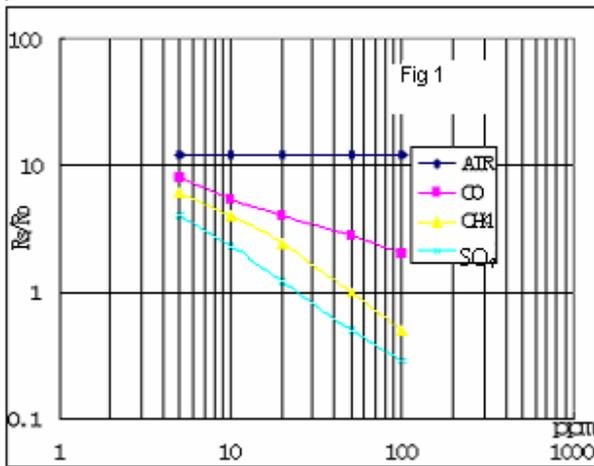
Fig.1 shows the typical sensitivity characteristics of the MQ136, ordinate means resistance ratio of the sensor ( $R_s/R_o$ ), abscissa is concentration of gases.  $R_s$  means resistance in different gases,  $R_o$  means resistance of sensor in 50ppm SO<sub>2</sub>. All test are under standard test conditions.
